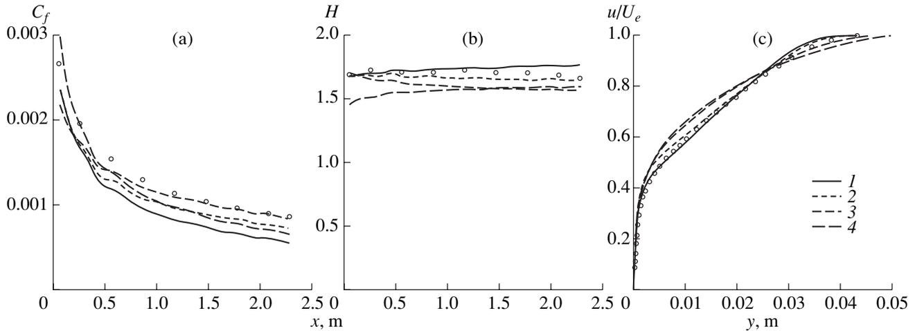
**Fig. 4.** Longitudinal distributions of the basic parameters of the boundary layer and the velocity profile for experiment 0241 [12]: (a) friction coefficient  $C_f$ , and (b) form factor  $H$ , (c) velocity profile at  $x = 1.168$  m. Notation is the same as in Fig. 1.
