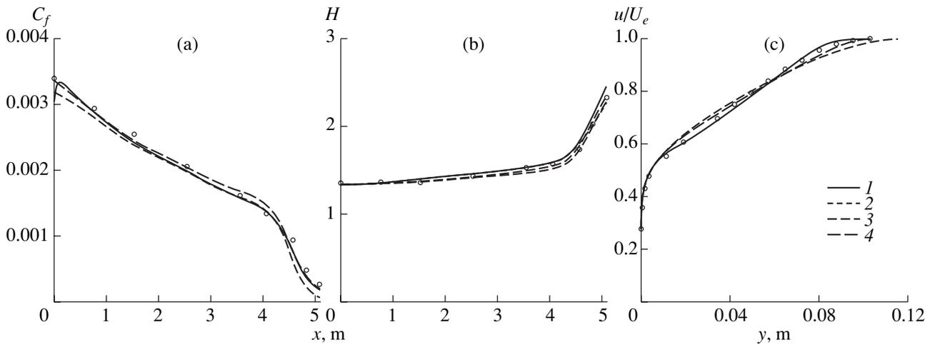
**Fig. 1.** Longitudinal distributions of the basic parameters of the boundary layer and the velocity profile for experiment 4800 [10]: (a) friction coefficient  $C_f$ , (b) form factor  $H$ , and (c) velocity profile at  $x = 3.556$  m. Calculation (1) by our model (relations (4)–(7), (12), (23), (24)), (2) by the algebraic model of [2], (3) by the Spalart–Allmaras model [13], and (4) by the Menter model [14]; dots indicate the experimental data of [10].
