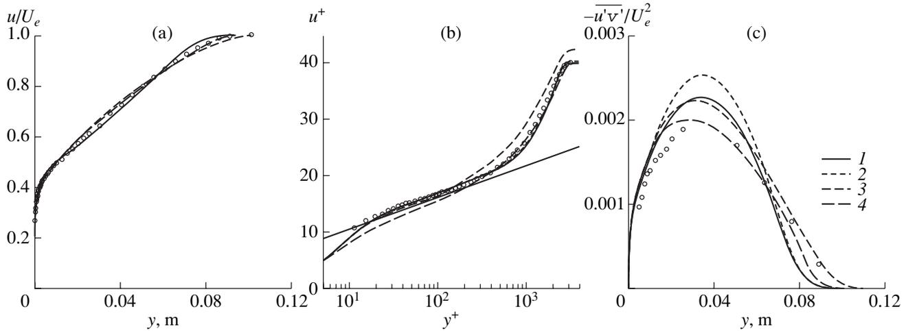
**Fig. 2.** Calculated and experimental velocity profiles and shear stresses for experiment 0141 [11] at  $x = 3.4$  m: (a) velocity profile in physical variables, (b) velocity profile in variables of the law of the wall, and (c) profile of shear turbulent stress  $\overline{u'v'}$ . Notation is the same as in Fig. 1.
