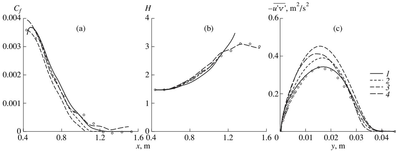
**Fig. 3.** Longitudinal distributions of the basic parameters of the boundary layer and the profile of shear turbulent stress for experiment DF [3]: (a) friction coefficient  $C_f$ , (b) form factor  $H$ , and (c) shear stress at  $x = 0.931$  m. Notation is the same as in Fig. 1.
